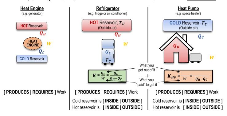
EXAMPLE: A heat pump has a coefficient of performance of 3.6 and a power supply of 7×10<sup>3</sup> W. Calculate the heat energy delivered into a home over 4 hours of use.
