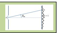
EXAMPLE: A 450 nm laser is shown through a single slit of width 0.1 mm. If the screen is a distance of 140 cm away from the slit, how wide is the central bright spot?
