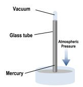
EXAMPLE: A classic barometer (as shown above) is built with a 1.0-m tall glass tube and filled with an unknown liquid.
