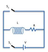
• CURRENT GROWTH: Current starts from [ ZERO | MAX ]; inductor resists growing current, eventually reaches \_\_\_\_
