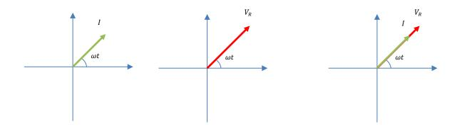
• Voltage across a resistor is IN PHASE with the current
