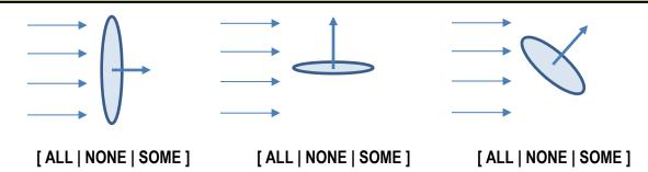
• ELECTRIC FLUX depends upon the ANGLE of the surface
