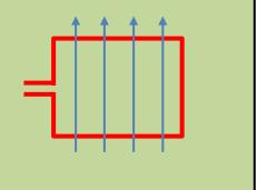
EXAMPLE: A loop with a magnetic moment of 0.5 Am<sup>2</sup> carries a current of 0.01 A. If it is placed in the presence of a magnetic field of strength 0.05 T, which points in the plane of the loop, what magnitude torque will the loop experience?
