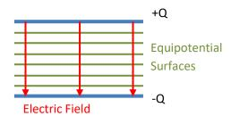
EXAMPLE: A parallel plate capacitor has an area of 5 cm<sup>2</sup>, a plate separation of 10 mm, and a voltage across the plates of 100 V. a) What is the charge of the capacitor? b) What is the magnitude of the electric field between the plates?
