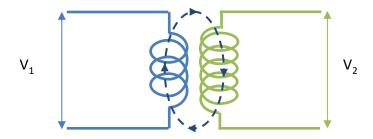
• The ratio of the VOLTAGES in a transformer depends upon the ratio of the TURNS:
